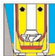
Sealing pot is open - the liquid is pumped off.
